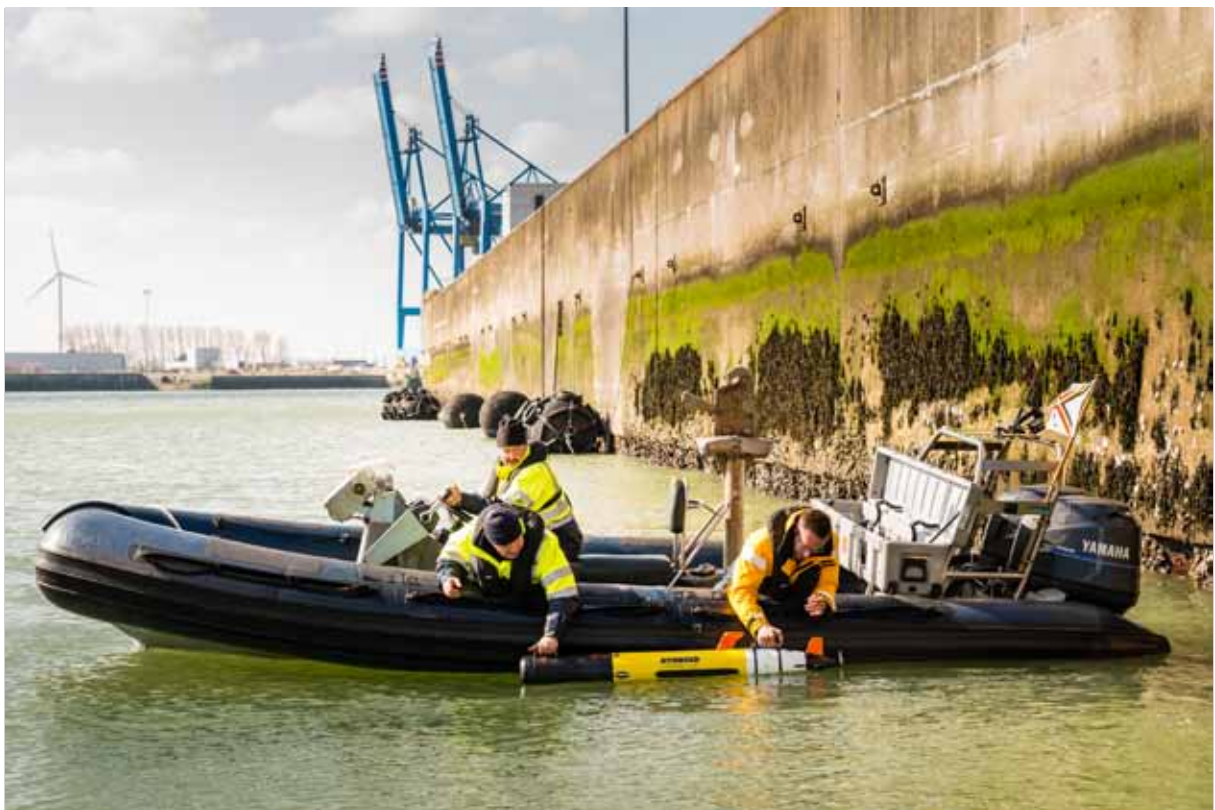
A REMUS Unmanned Underwater Vehicle can be deployed for demining ports and shallow waters, both nationally and during expeditionary operations.
