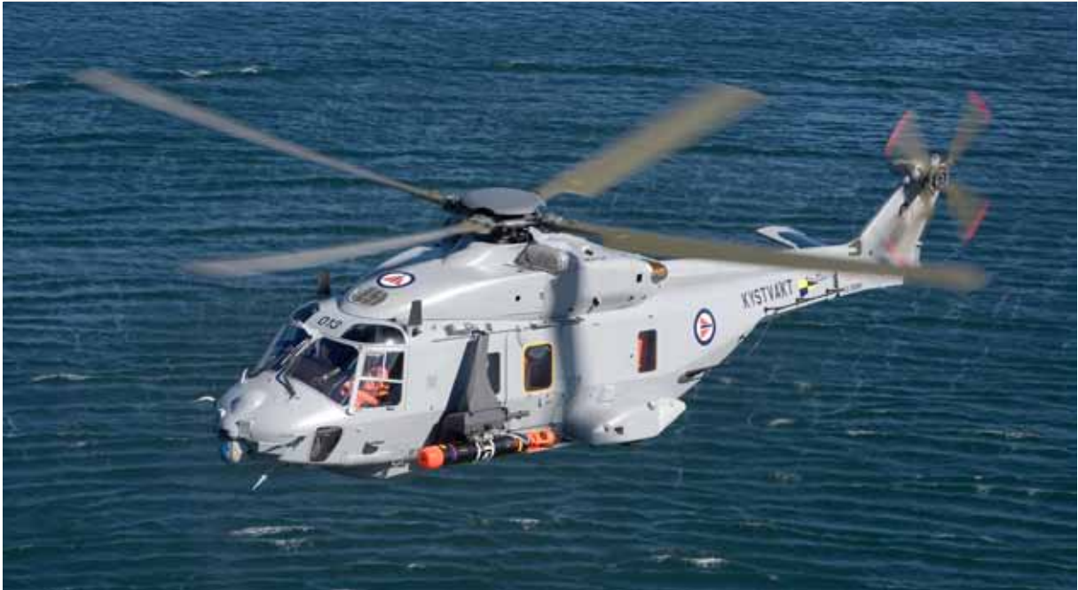
A sonar and torpedoes turn the maritime NH90 helicopter into a maritime combat capability that can be deployed from a frigate for anti-submarine warfare.
