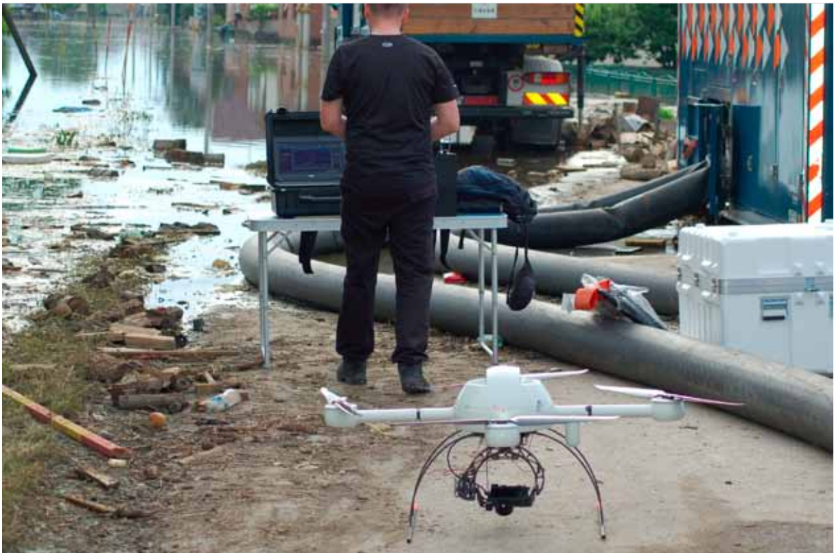
Floods in Bosnia and Herzegovina in May 2014 washed away mines of uncleared minefields. B-FAST used drone technology developed by the Royal Military Academy to map the dissemination of the explosive ordnance.
